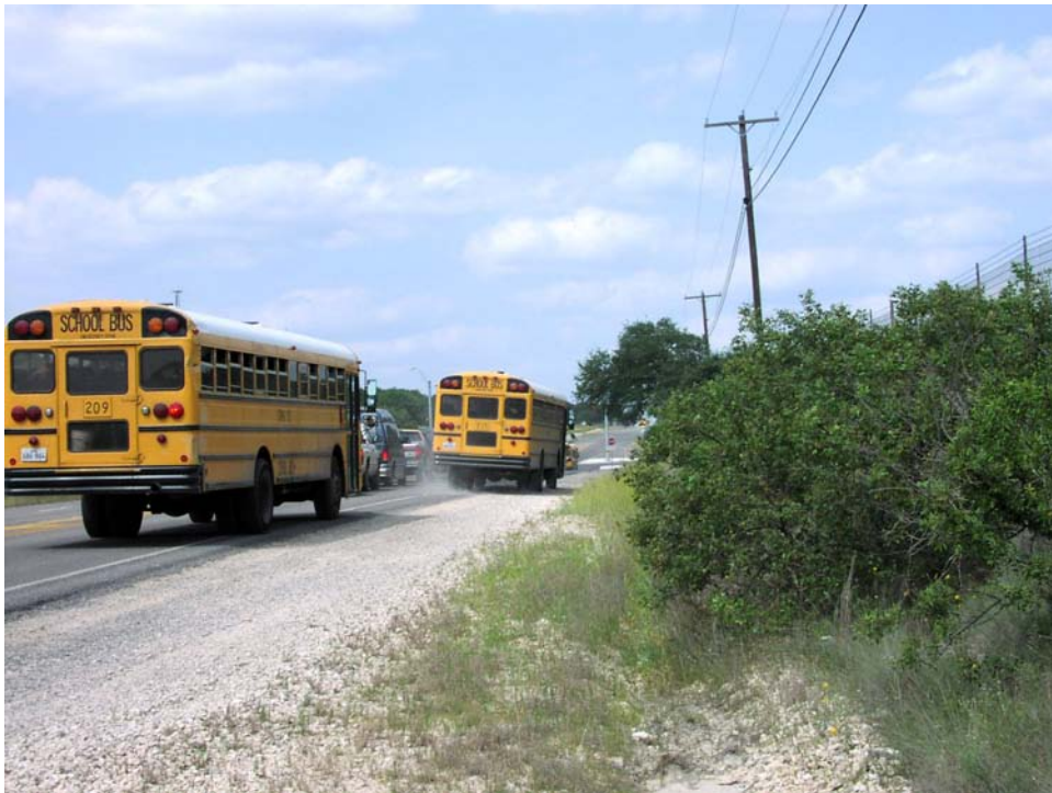
Figure 7-210. Buses Using the Gravel Shoulder on the State Highway to Bypass the Queue Length on the FM Road Created by Northbound Traffic.
